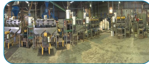
Flotation Pilot Plant Operation at ALS, Perth
